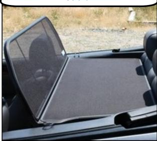
Once in installed your wind deflector is held in place by two spring plungers in the back and two brackets in the front. (There are also two straps which aren't shown in the photos below)
