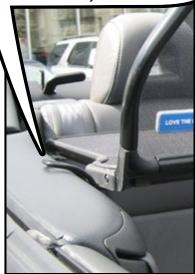
Step 1: Your wind deflector attaches to the small holes in the rear trim panel. There are two "L" handled spring plungers. The "nose" of the plungers will go into the holes. Start with the plungers in the closed position as shown in the top right photo.
