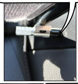
Step 4: The two front brackets will rest o the top of the trim panel.
